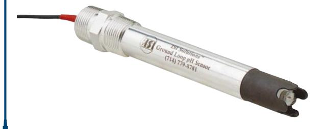
The HPW pH sensor is designed to meet ASTM standard D5128-90 guidelines for successful measurement of pH in high purity water. Sensor features include a stainless steel housing, TOP68 quick disconnect cable connector, differential preamplifier, low impedance glass pH electrode and porous Teflon® double junction reference cell with KCI/AgCI and KNO³ electrolyte.
