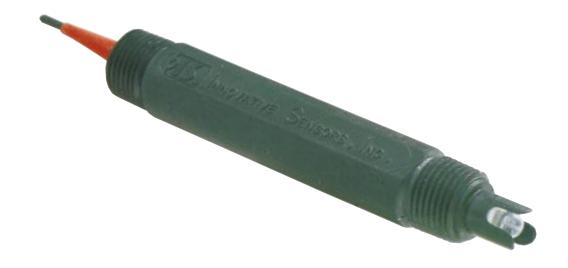
The Model 25 pH sensor features 1/2" MNPT threads for insertion, peripheral porous Teflon® liquid junction, double junction reference cell, solution ground, 3.3M (10.0 ft.) cable with BNC connector. Typical applications include wastewater treatment, cooling towers, plating baths and general industrial service.
